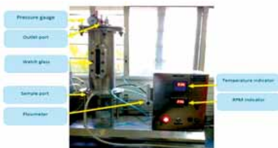
Fig. 3: Bench scale fermentation set up for syngas fermentation experiments
