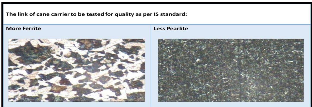
Fig. 2: Microstructure of more Ferrite and Less pearlite materials
